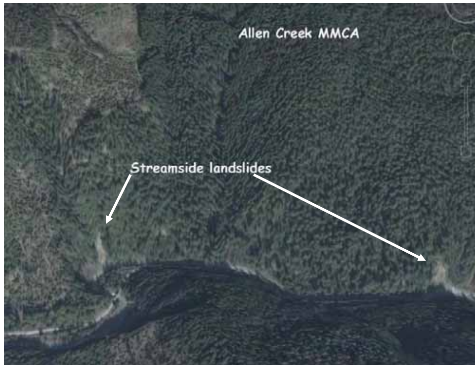
Photo 5-7. Streamside Landslides along Yager Mainstem Canyon Reach.
