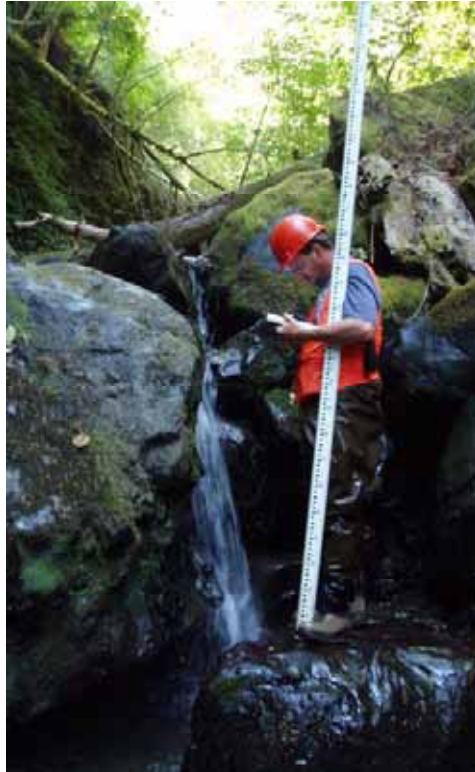
Photo 5-27. A 7.7-foot High Bedrock/Boulder Fish Barrier in Beer Bottle Creek.
