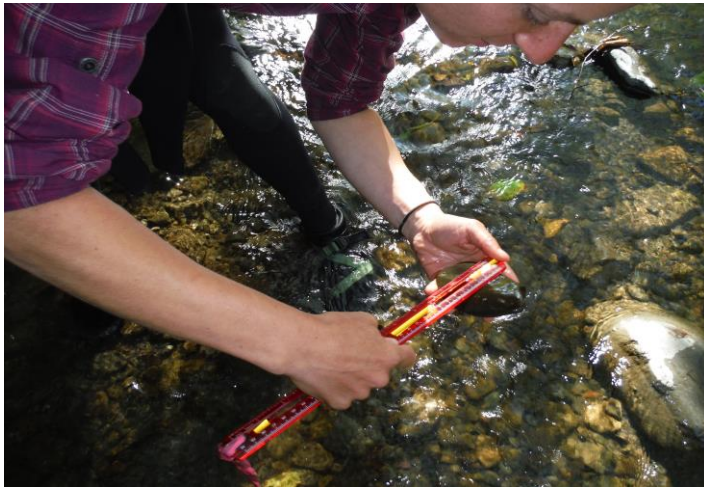
Figure 3. Measuring particle size (mm) of the streambed surface
