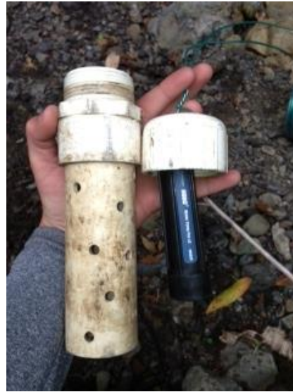
Figure 8. Stream temperature logger with protective PVC case
