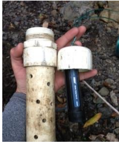
Figure 8. Stream temperature logger with protective PVC case
