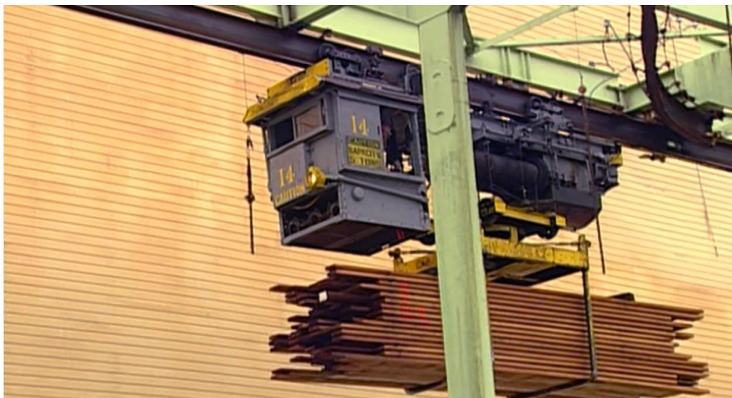
Figure 11 Monorail I-beam rail, prototypical trolley/ car, photo date unknown.
