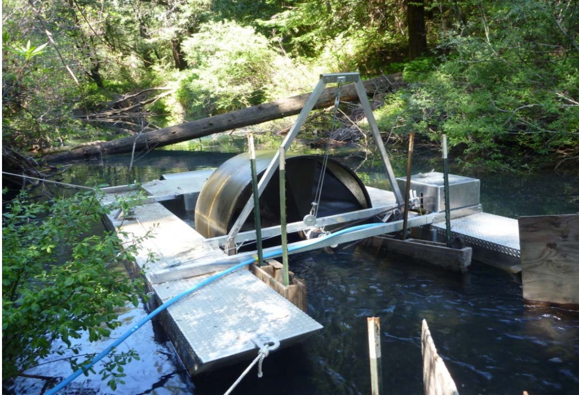
Figure 1. A motorized rotary screw trap in the North Fork Navarro River 2015.
